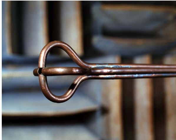
Fig. 7. Broadband, high intensity point noise source consisting of four impinging air jets.
