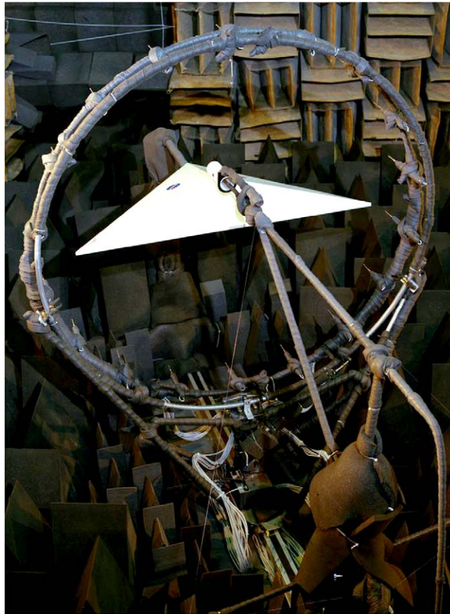
Fig. 1. Photograph of wedge-shape airfoil model experiment set-up in anechoic chamber, view looking upstream.
